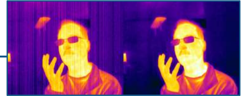
Raw image (left) and image after applying filter developed with HDL Coder (right).
